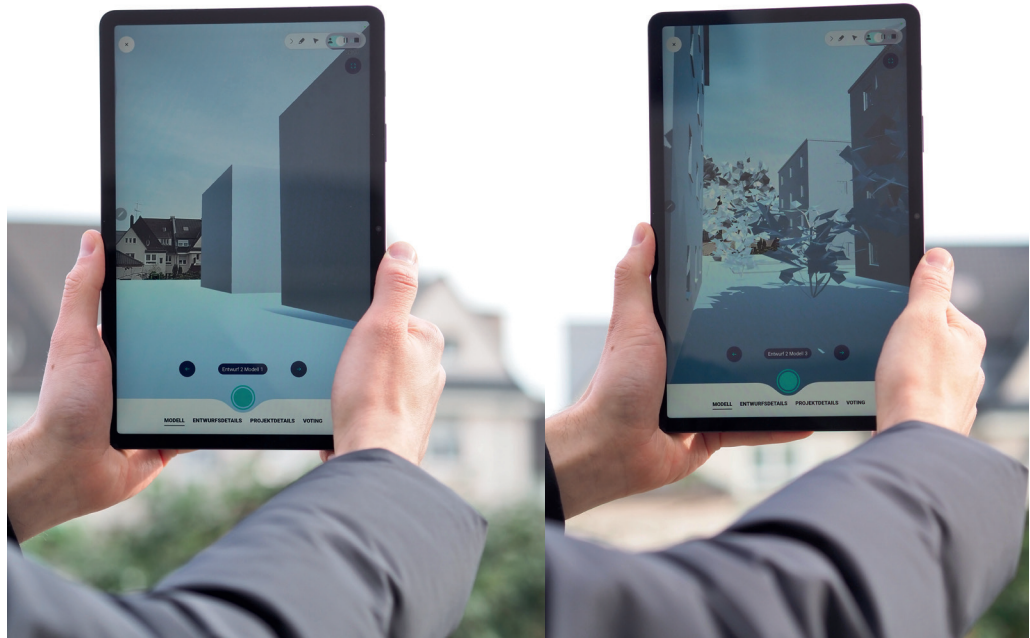
Fig. 6 – In situ visualisation of urban designs as 3D model in LOD 1.1. and LOD 3.3. via augmented reality in the City of Schwerte. Source: TU Dortmund University - Department of Spatial Planning - Research Group of Urban and Regional Planning, Luisa Nagel, 2024.
